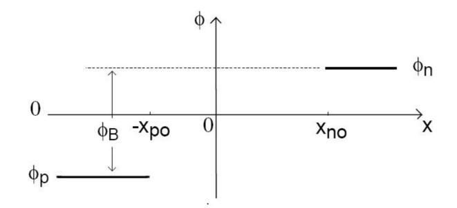
$$\phi_p = -V_{th} \ln \frac{p_o}{n_i} \stackrel{\uparrow}{=} -V_{th} \ln \frac{N_A}{n_i}$$
