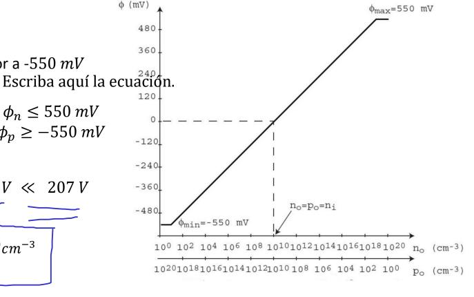
$\phi_{B_{MAX}} = 277 \, mV \, - (-550 \, mV) = 827 \, mV \ll 207 \, V$
